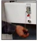
13. Operate Pepper Spray Port 1) Open inner door just enough to insert hose. 2)Unscrew cap, insert nozzle, spray. 3) Replace port cap when finished.
